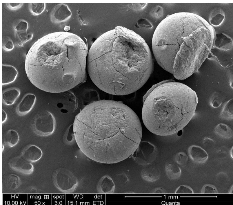
Fig.- SEM picture of Sodium Alginate microspheres (high magnification)
